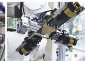
組入扣環 Circlip press fit by robot
