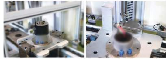
粉塵清潔 Dust cleaning the stator and the internal body
