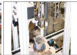
檢測扭力值 Inspect screw tighten torque
