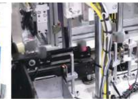
矽鋼片厚度檢測 Lamination thickness detection
