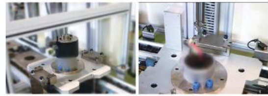
粉塵清潔 Dust cleaning the stator and the internal body
