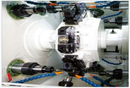
0° / 90° / 180° 三方向刀具佈置 Tri-directional (0°/90°/180°) tool configuration
